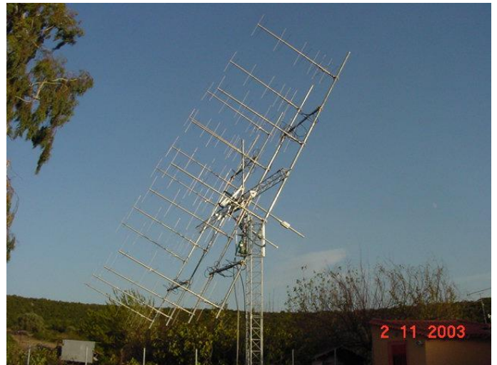
SV1BTR used this array of Yagis on 2 meters to make 24 CW QSOs off the Moon. (Photo by SV1BTR)
